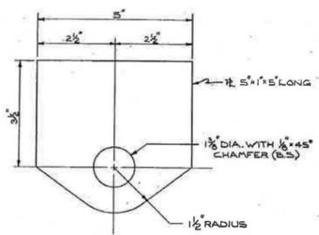
CONDUCTOR ATTACHMENT PLATE (MANUFACTURER MAY SUBMIT ALTERNATE TO ACCOMMODATE ARM.)
